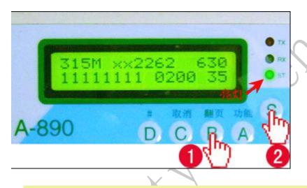
Power on, display the main menu (A890-RES 3&4M),RX lights flashing indicates entry into the receiving State, received
